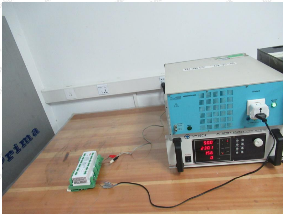
Photo of Flicker/ Harmonic Test
