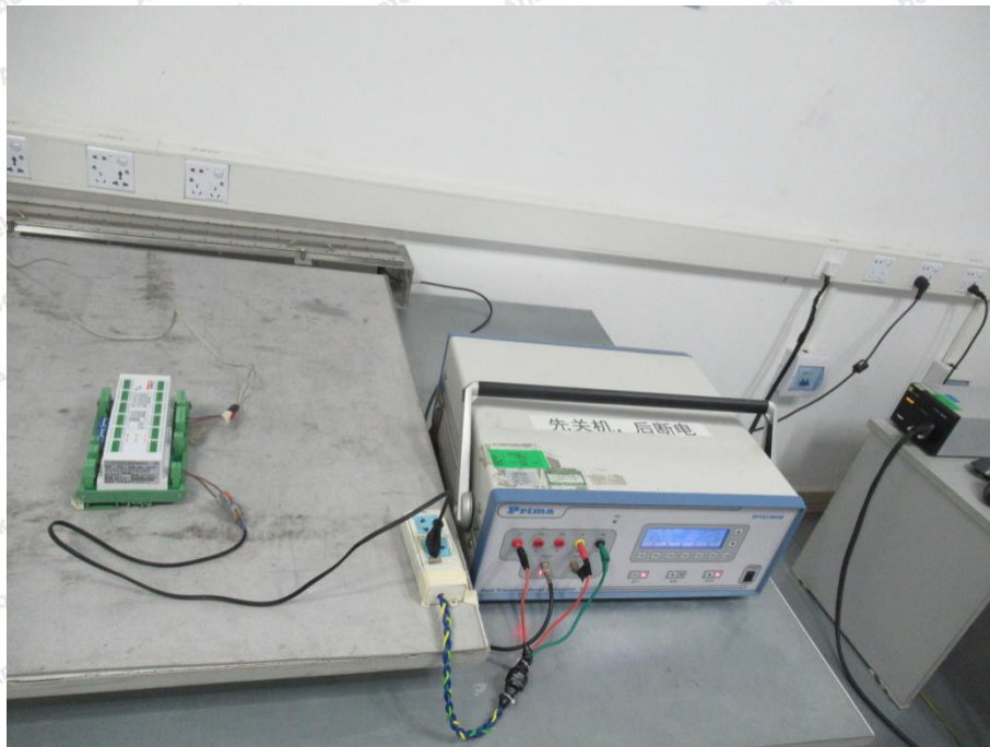
Photo of Electrical Fast Transient/Burst Immunity Test
