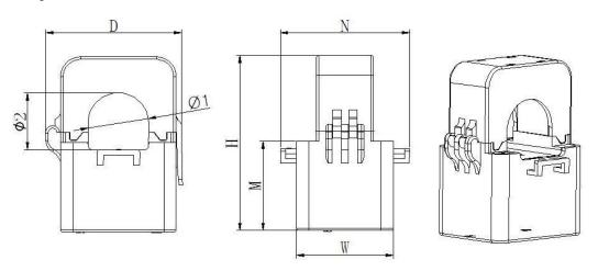
Note: Primary current flow from P1 to P2. The black second wiring is S2, the red is S1. The outlet length is  $1m \pm 10$ cm.
