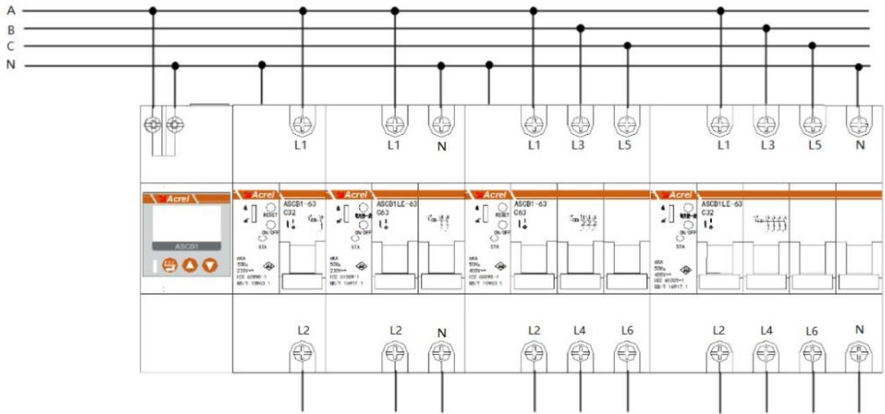
Figure 5 Installation and wiring example diagram
