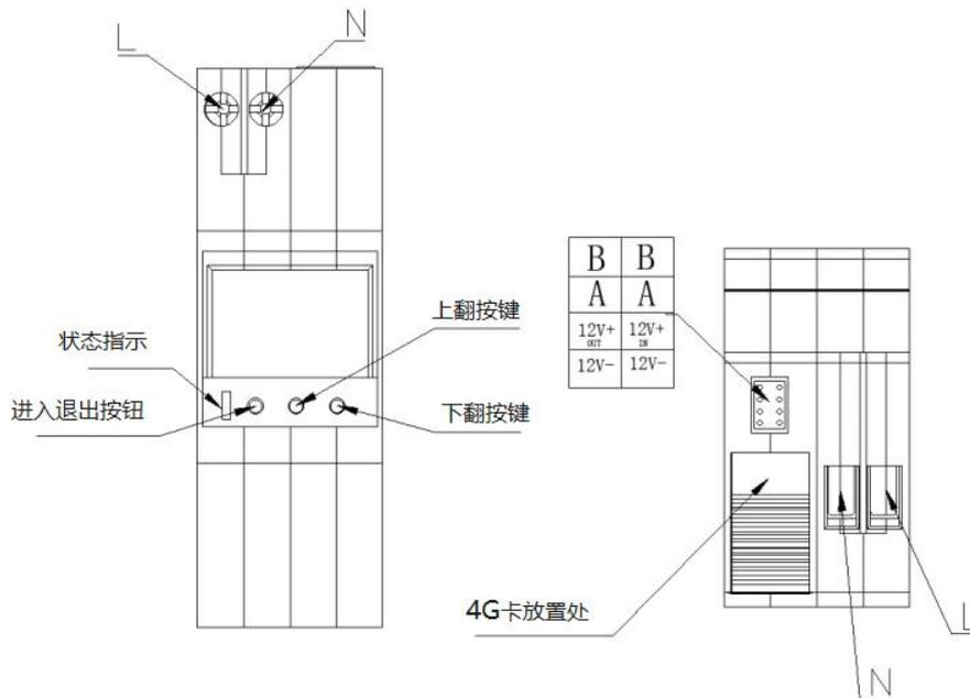
Figure 4 Schematic diagram of smart gateway wiring terminals
