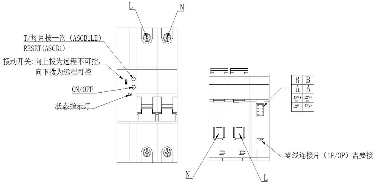
Figure 2 Schematic diagram of intelligent miniature circuit breaker wiring terminal
