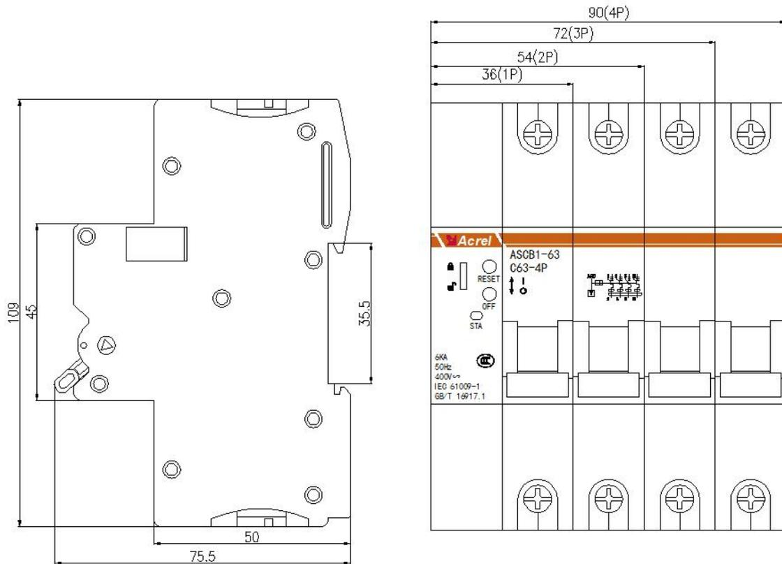
Figure 1 Outline dimension drawing of intelligent miniature circuit breaker
