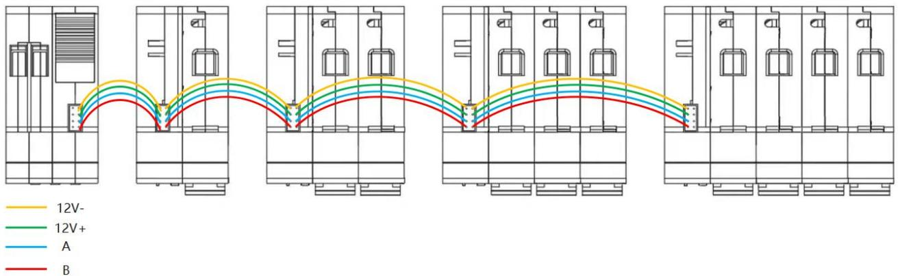
Figure 7 Schematic diagram of 4pin terminal wiring (top view)
